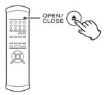
Pressing OPEN/CLOSE opens the tray if it is closed, and closes it if it is open. When the tray is opened during playback, it may take a few seconds before the disc is "unloaded" and the tray opens.
